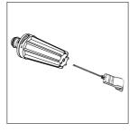
A clogging up in the nozzle causes a pump pressure which is too high. This is why cleaning is required immediately.
